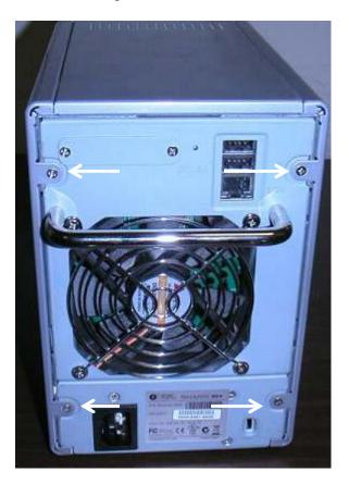
Next, remove the 4 screws that connect the power supply to the ReadyNAS. There will be 2 screws on the left and 2 on the right to remove the power supply. You can disregard the sticker that says "warranty void if this tag broken".
