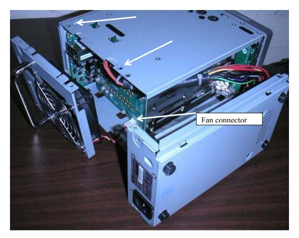
The power supply cable will be connector should be in full view now. You will need to hold down the clip while pulling out the cable to remove the power supply.
